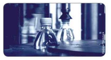
**Continuous Production** uses a highly automated manufacturing system to meet the demands of a worldwide market. Machinery and production lines are continuous, sometimes for 24 hours a day. The set up and running costs are high but economies of scale offsets these costs. Typical products manufactured with this system include everyday use products like drinks bottles, screws, DVDs, and other products which don't change from year to year.
