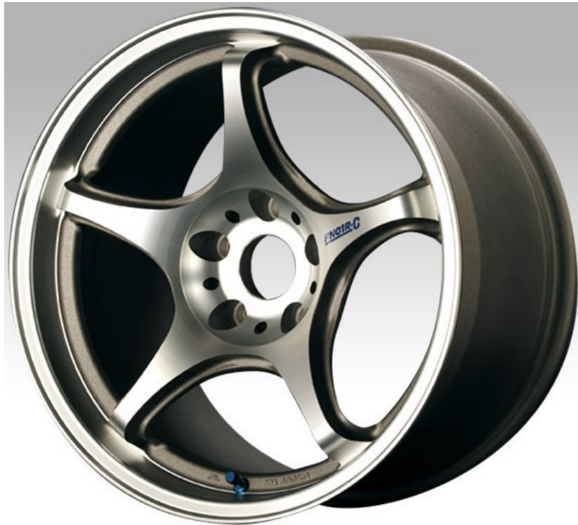
Sand cast aluminium car wheel rim after machine finishing
