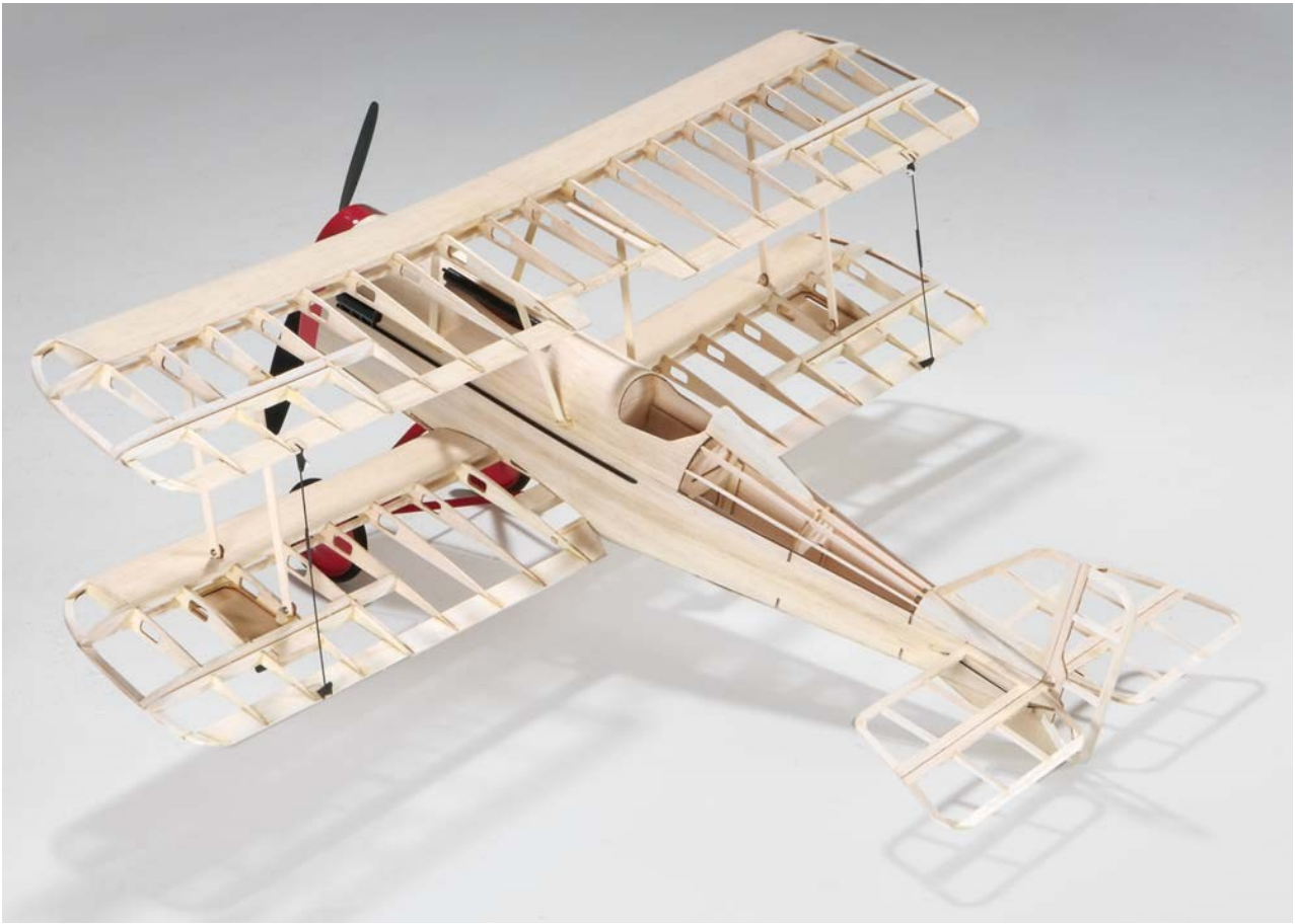
Model plane - lightweight balsa wood fuselage glued together before finishing with fabric
