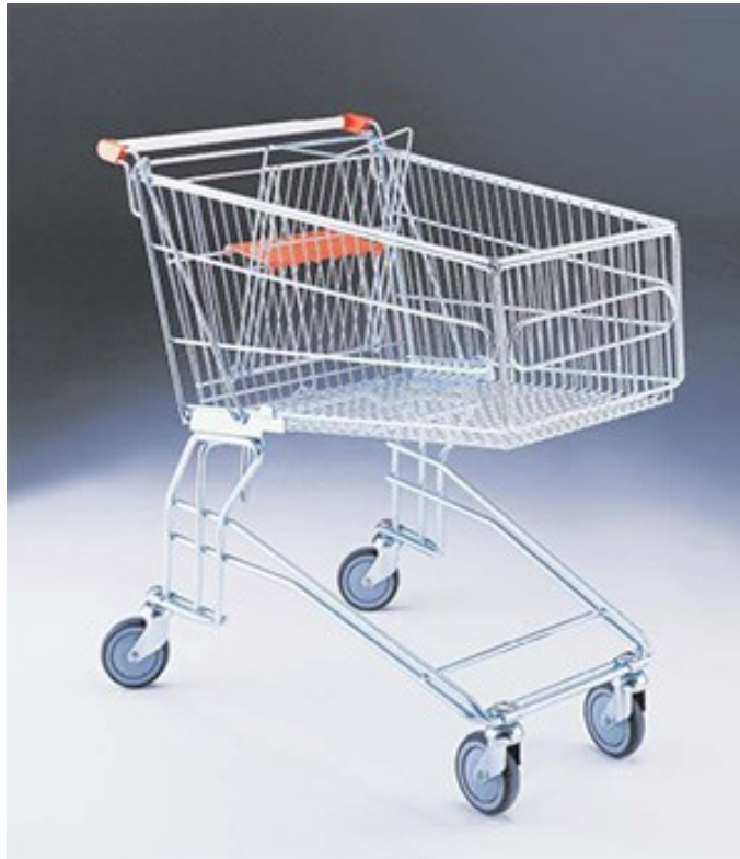
Solid mild steel rod shopping trolley welded construction and galvanised (zinc) finish
