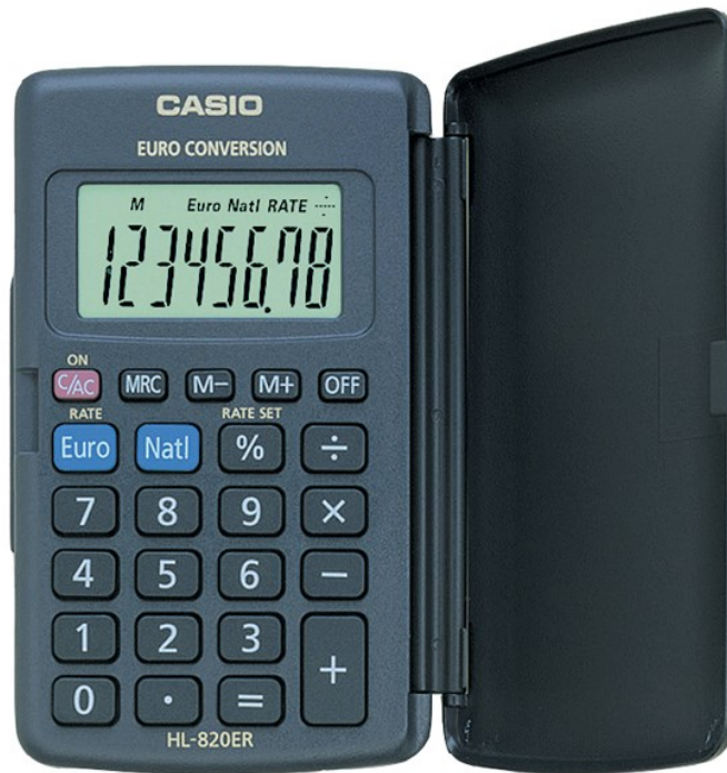
Calculator - injection moulded hinge and sliding battery lid, case screwed and copper battery contacts staked to the HIPS
