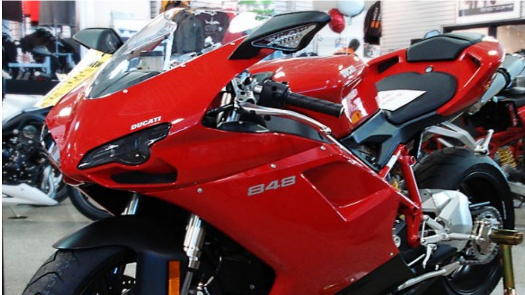
Ducati's motorbike screens and light lens - compression moulded from acrylic
