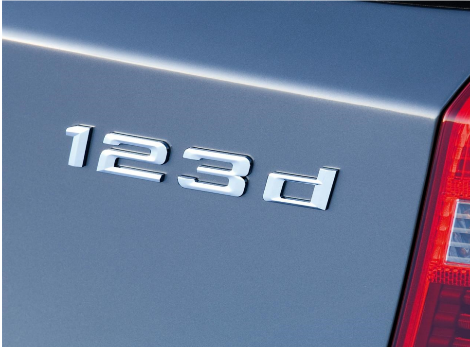
BMW's chromed ABS decal glued onto the painted steel boot panel
