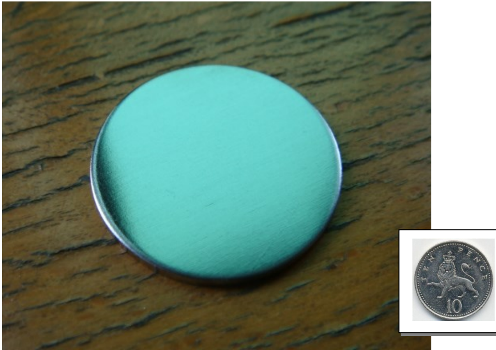
Nickel alloy blank which will be embossed to form a 10p coin
