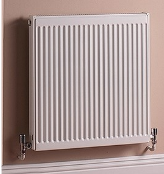
Pressed steel panels spot welded to form a central heating radiator
