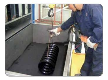
The process involves the degreased and clean metal being heated to approximately 180°C before **fluidisation** (coating process) takes place in a special tank. The metal object is then submerged quickly into the fluidised powder and left for a few seconds, enabling the powder to stick to the metal in the form of a thin coating. The object is then returned to the oven to allow the coating to fuse and leave a smooth glossy coating.
