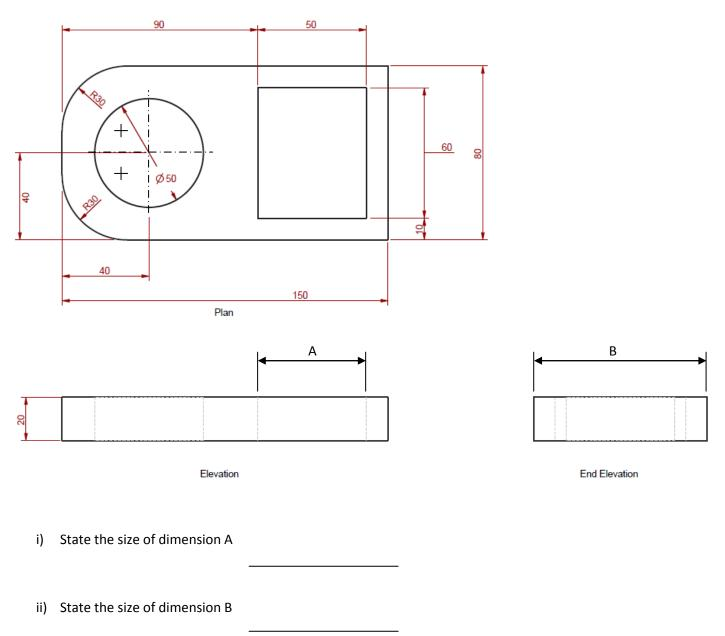
iii) There are 4 mistakes with the dimensions on the Plan of the cup holder. Circle each of these mistakes.
