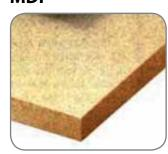
MDF is a relatively cheap board of good quality. This board is composed of fine wood dust and resin pressed into a board. This material can be worked, shaped and machined easily. Paint can be applied to it without the need for an undercoat or primer.
