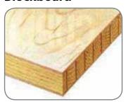
Blockboard is built up with numerous strips of softwood sandwiched between two sheets of hardwood on the top and bottom and glued together under high pressure.
