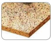
Chipboard is made up of wood particles including chips, shavings and sawdust from all different types of commercial timber glued together under heat and pressure.
