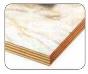
Plywood is built up of odd numbers of thin layers (veneers) of hardwood or softwood called laminates, with each one running at 90 degrees to each other. The layers are glued together by an adhesive and pressure applied.
