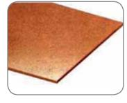
Hardboard is made from wood fibres obtained from chips and pulped wood waste. The pulp is put under pressure until the fibres bond to produce a tough board that is smooth on one side and rough on the other.
